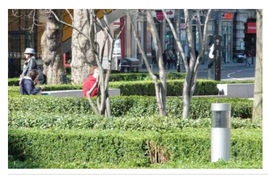
1 and 2: Areas of planting can provide attenuation of rainfall, preventing its rapid transit to conventional drains. For example, this improvement scheme at St Paul's incorporates soakaways.
