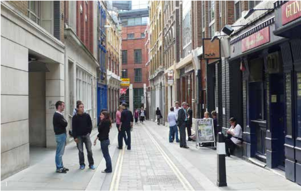
1: Raised carriageways, where the carriageway is raised to footway level, are a useful tool for providing a more comfortable and accessible walking environment.
