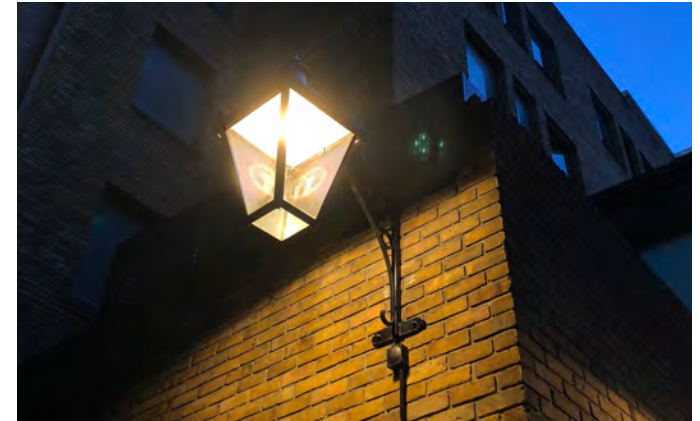
Discharge lamp period style lantern fitted with appropriate LED module
