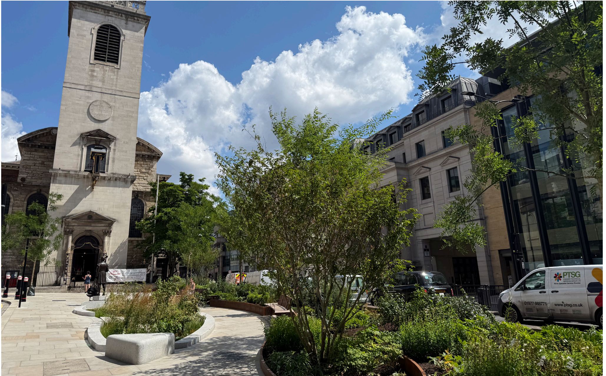
Little Trinity Lane: Flood resilience at Little Trinity Lane, which captures surface water running down Garlick Hill storing it in the beds to irrigate plants.
